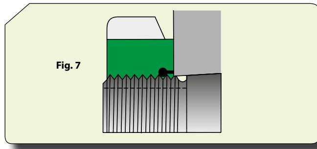
*Bearings fitted on withdrawal sleeves must rest against a fixed shoulder on the shaft and the sleeve is fitted subsequently and pressed into the tapered bore of the bearing.*
