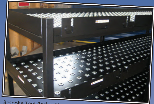
Bespoke Tool-Rack with sunk Ball Transfer Units
